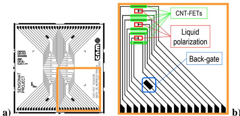
Figure S1. a) Schematic of  $0.5 \times 0.5 \text{ cm}^2$  chip platform. b) Elements on a quadrant: 6 CNT-FET structures, back-gate electrode and 3 liquid polarization electrodes and 16 pad matrix.
