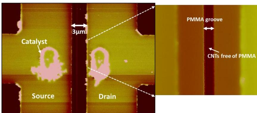
Figure S2. A closer look of the source and the drain electrodes after they had been passivated with PMMA. A zoom of the 500 nm groove on the PMMA layer is also shown.
