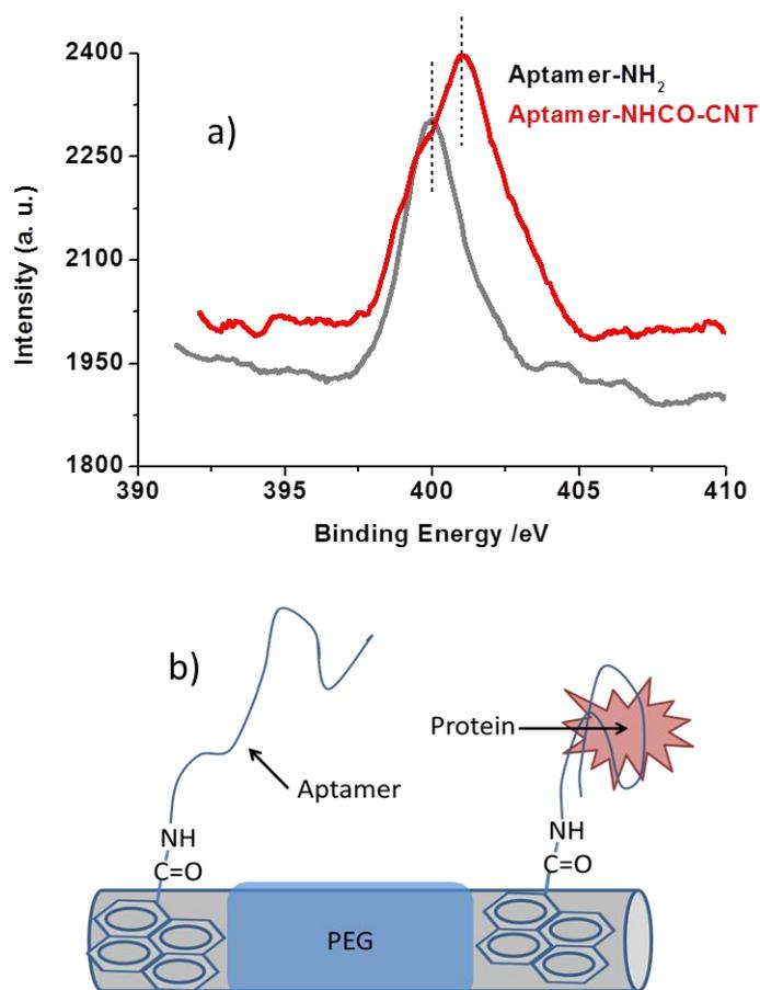
Figure S4. a) XPS spectra of the aminated aptamer and the amide formation on the pyrene modified CNT. b) Scheme showing the functionalized carbon nanotube.
