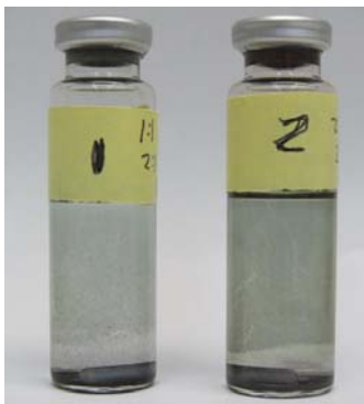
Figure S5. Representative solutions of [\text{PPh}_3]/[\text{AgNO}_3] = 1.0 (vial 1) and 2.0 (vial 2) at t \approx 48 h after \text{NaBH}_4 addition. Further solution phase processing in the Ag- \text{PPh}_3 systems results in larger silver species, indicated by the dark grey sediment at the bottom of both vials. Sedimentation is not observed in any Ag- \text{L}^n solutions examined.
