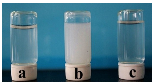
Fig. S3. Photographs of (a) single-component \text{Pb}(\text{NO}_3)_2 solution at pH 4.0 and (b) white precipitate obtained by adjusting pH value of single-component \text{Pb}(\text{NO}_3)_2 solution to 6.0. (c) Photographs of PAH/ \text{Pb}(\text{NO}_3)_2 mixture solution at pH 6.0.
