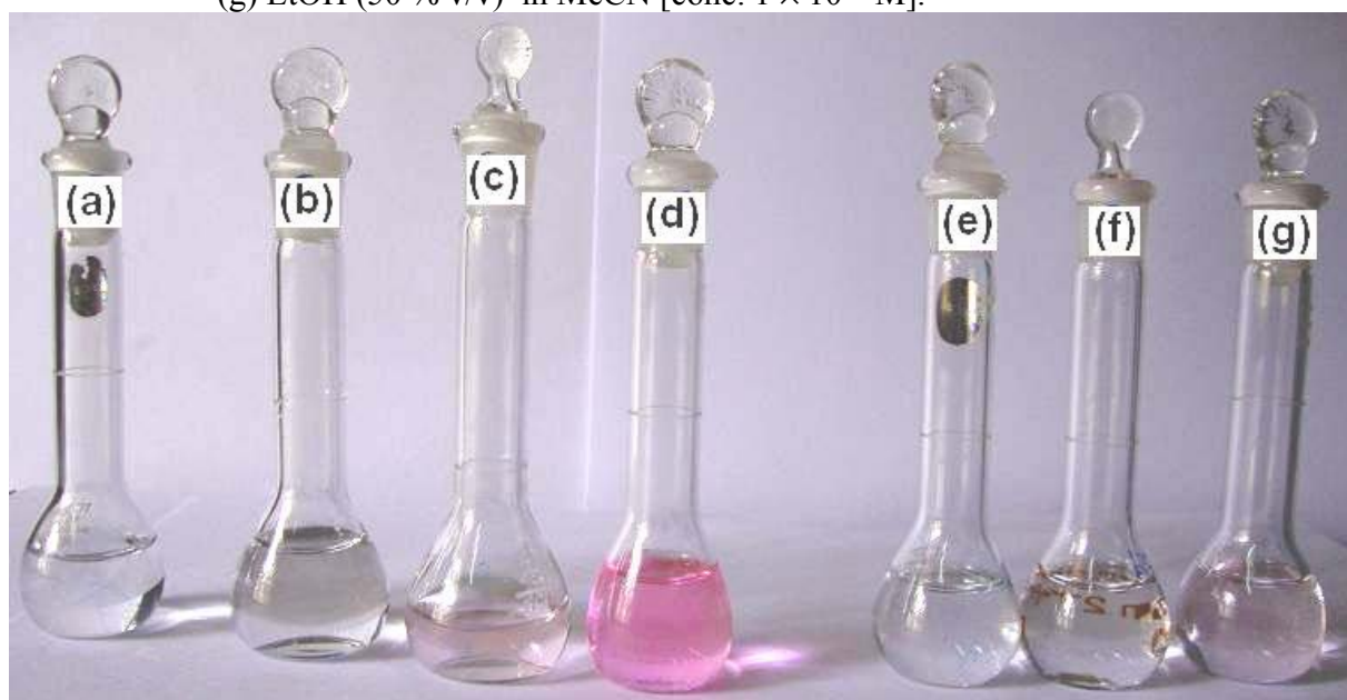
Figure S30. Photographs of 3 alone (a) and in presence of (b) MeOH (10 % v/v), (c) MeOH (30% v/v), (d) MeOH (50 % v/v), (e) EtOH (10 % v/v), (f) EtOH (30 % v/v) and (g) EtOH (50 % v/v) in THF [conc. 1 \times 10^{-6} M].
