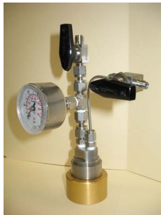
Fig. S2. Pressure vessel with a multi-port lid used for AFEX
