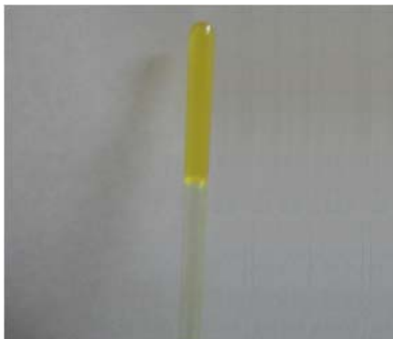
Fig 9S. Photograph of Receptor 1 ( c = 3.58 \times 10^{-3} M) with 5 equiv. amounts of Fluoride ( c = 1.5 \times 10^{-2} M) in DMSO.
