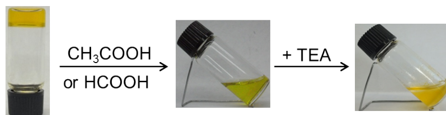
Figure S13 The irreversible gel-sol transitions of organogel ( 1a /cyclohexane) triggered by \text{CH}_3\text{COOH}/\text{HCOOH} -TEA stimuli.
