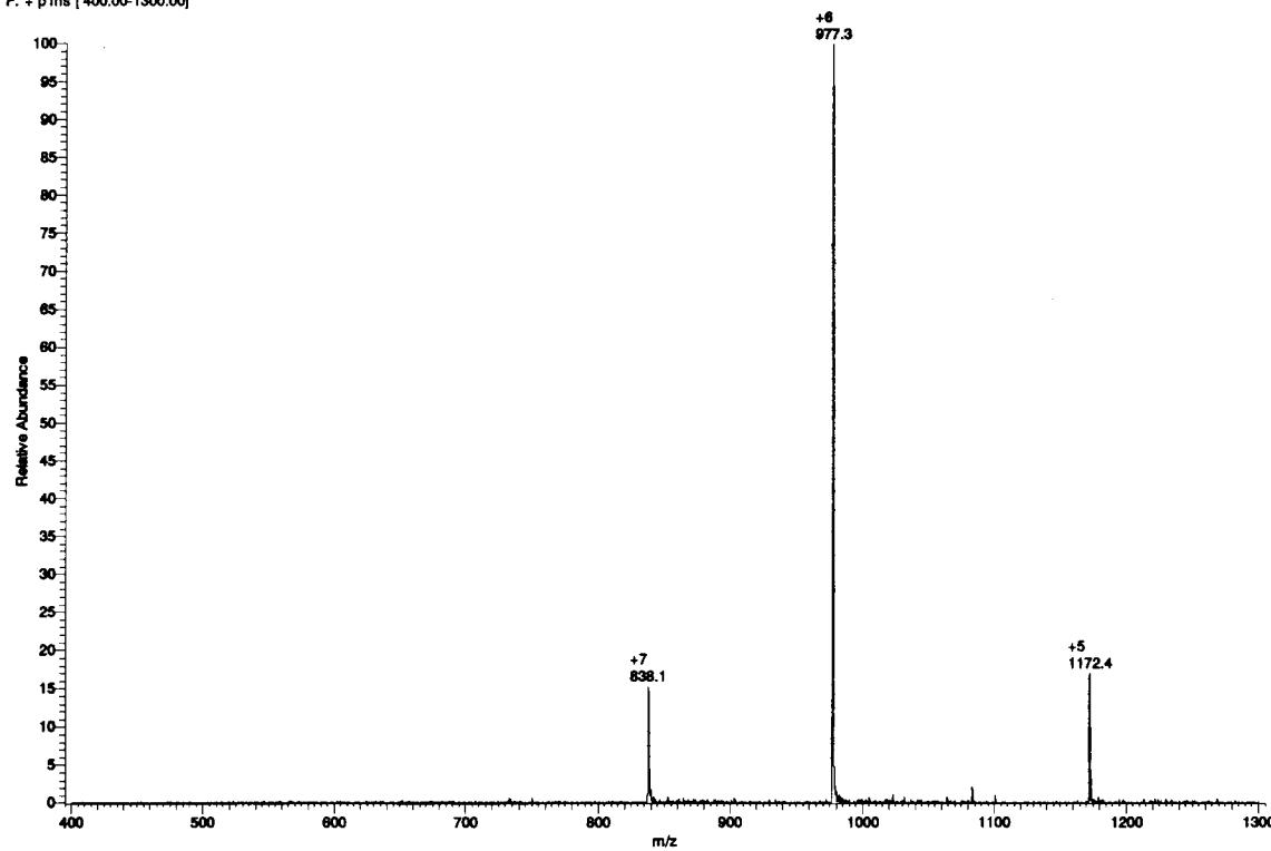
The mass of metastin was determined by electrospray mass spectrometry using a ThermoFinnigan LCQ ion trap mass spectrometer (ThermoQuest, U.S.A.). Sample was dissolved in 1% formic acid-50% acetonitrile.
