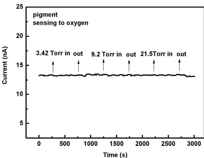
The oxygen-sensing of azo pigment with irradiation of 370 nm light is revealed. Various partial pressures of oxygen injections and extractions are shown by arrows.
