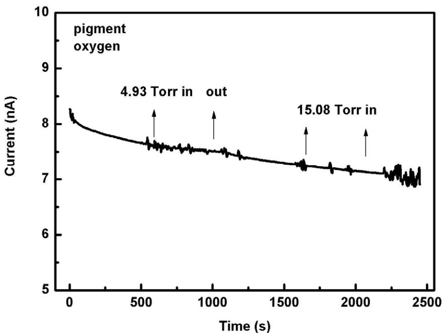
The oxygen-sensing of azo pigment without irradiation of 370 nm light is revealed. Various partial pressures of oxygen injections and extractions are shown by arrows.
