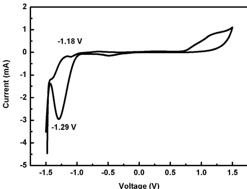
Cyclic voltammetry curve of azo pigment in the solution of DMF with 0.2 mol/L TBAP. The reduction potential of azo pigment is -1.47 V vs NHE (-1.23 V vs Ag/AgCl). The reduction potential of azo pigment is corresponding to its LUMO, whose energy level is -3.2 eV (vs vacuum). Actually, the LUMO also is the  $\pi^*$  orbit.
