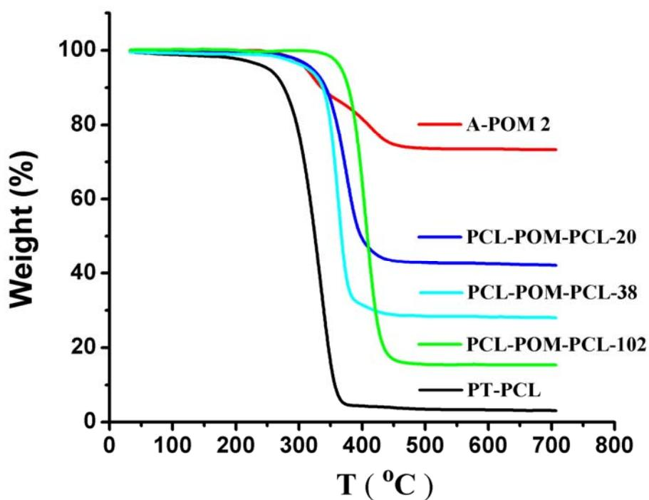
Figure S18. TGA thermograms of A-POM 2, PT-PCL and PCL-POM-PCL hybrids.
