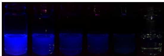
Figure S3. Photographs of PFBI solutions with different concentration of \text{Cu}^{2+} . (a) 0 M (b) 1.0 \times 10^{-5} M (c) 2.5 \times 10^{-5} M (d) 5.0 \times 10^{-5} M (e) 7.5 \times 10^{-5} M (f) 1.0 \times 10^{-4} M.
