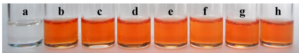
Figure S10: Photograph of L2 solution ( 2.5 \times 10^{-5} \text{M} ) in DMSO after the addition of 1 equiv. of tetrabutylammonium fluoride and 1 equiv. of other anions. (a) Free Receptor L2, (b) \text{F}^- , (c) \text{Cl}^- + \text{F}^- , (d) \text{Br}^- + \text{F}^- , (e) \text{I}^- + \text{F}^- , (f) \text{NO}_3^- + \text{F}^- , (g) \text{HSO}_4^- + \text{F}^- and (h) \text{H}_2\text{PO}_4 + \text{F}^- .
