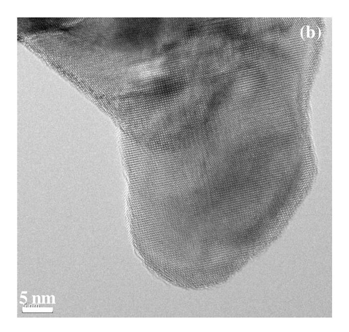
Figure SI1 HRTEM images of the (a) LNMO and (b) LCMO nanoparticles.
