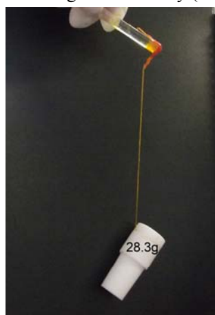
Fig. S3 The wire-drawing photograph of OSPCMs.
