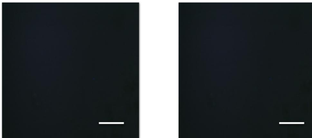
Figure S3. Fluorescent characterization of plasma oxidized (100 w, 20 min) PDMS with phage displayed peptides LSNNNLR (left) and LQPRANF (right). Scale bar: 50 \mu m.
