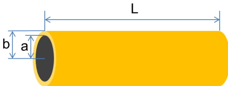
Figure S2. Schematic of a cylindrical rod covered by ferroelectric layer and surface electrode.
