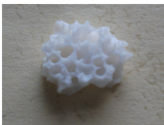
Fig. S1 Picture of hierarchical zeolite H-beta with a honeycomb-like monolith
