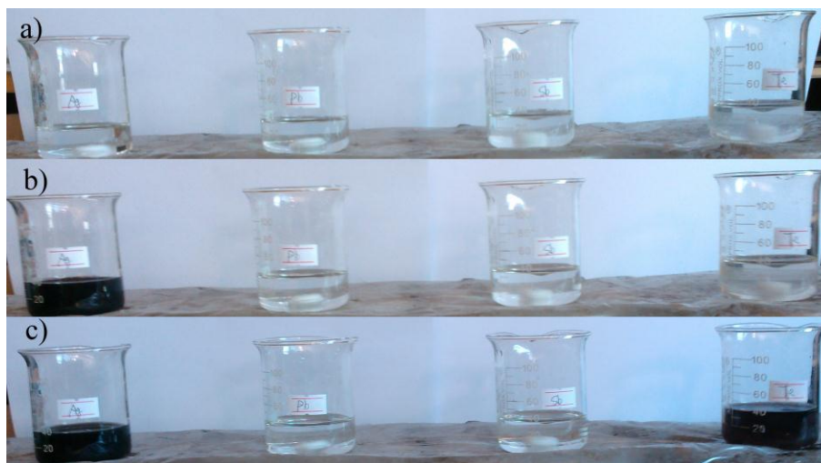
Figure S1 (a) the beakers with \text{AgNO}_3 , \text{Pb}(\text{CH}_3\text{COO})_2 \cdot 3\text{H}_2\text{O} , \text{K}(\text{SbO})\text{C}_4\text{H}_4\text{O}_6 \cdot 0.5\text{H}_2\text{O} , \text{Na}_2\text{TeO}_3 dissolved in mixture solvents of ethylene glycol and formamide, respectively. (b) the beakers with \text{N}_2\text{H}_4 added at the same time. (c) the beakers with time prolonging.
