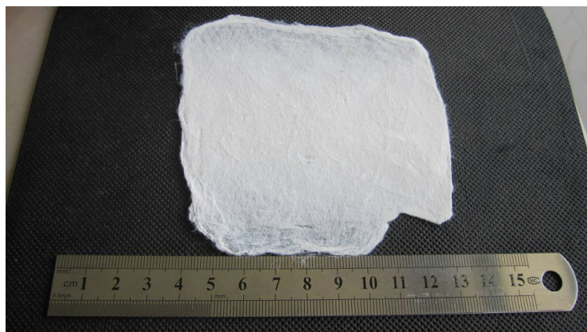
Fig. S4 Photograph of as-spun large iPP porous nonwoven mesh.
