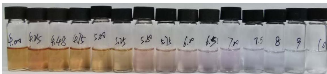
Fig. S17 Photo of probe 1 (50 \mu\text{M} ) in ACN-phosphate buffer (20 mM, 1:1, v/v) at various pH.
