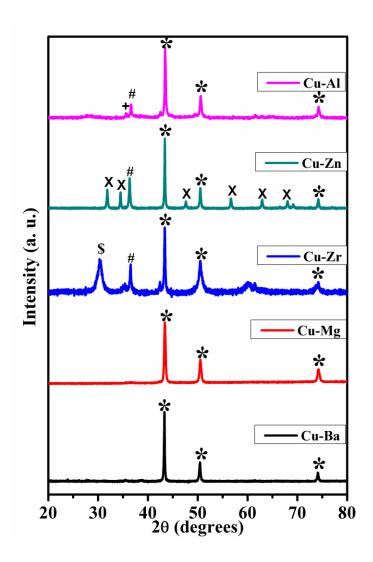
**Fig. 1** XRD patterns of different recovered copper catalysts. (\*)  $Cu^0$ , (#)  $Cu_2O$ , (+) CuO, (\$) t- $ZrO_2$ , (X) ZnO.
