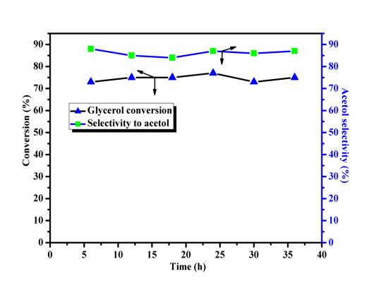
Fig. 2 Time on stream activity of Cu-Al catalyst.
