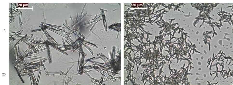
Fig. S4. Optical microscopy images (100x magnification) of: a) the microcrystals of 1; b) short fibrils formed after 3 min sonication of the microcrystals
