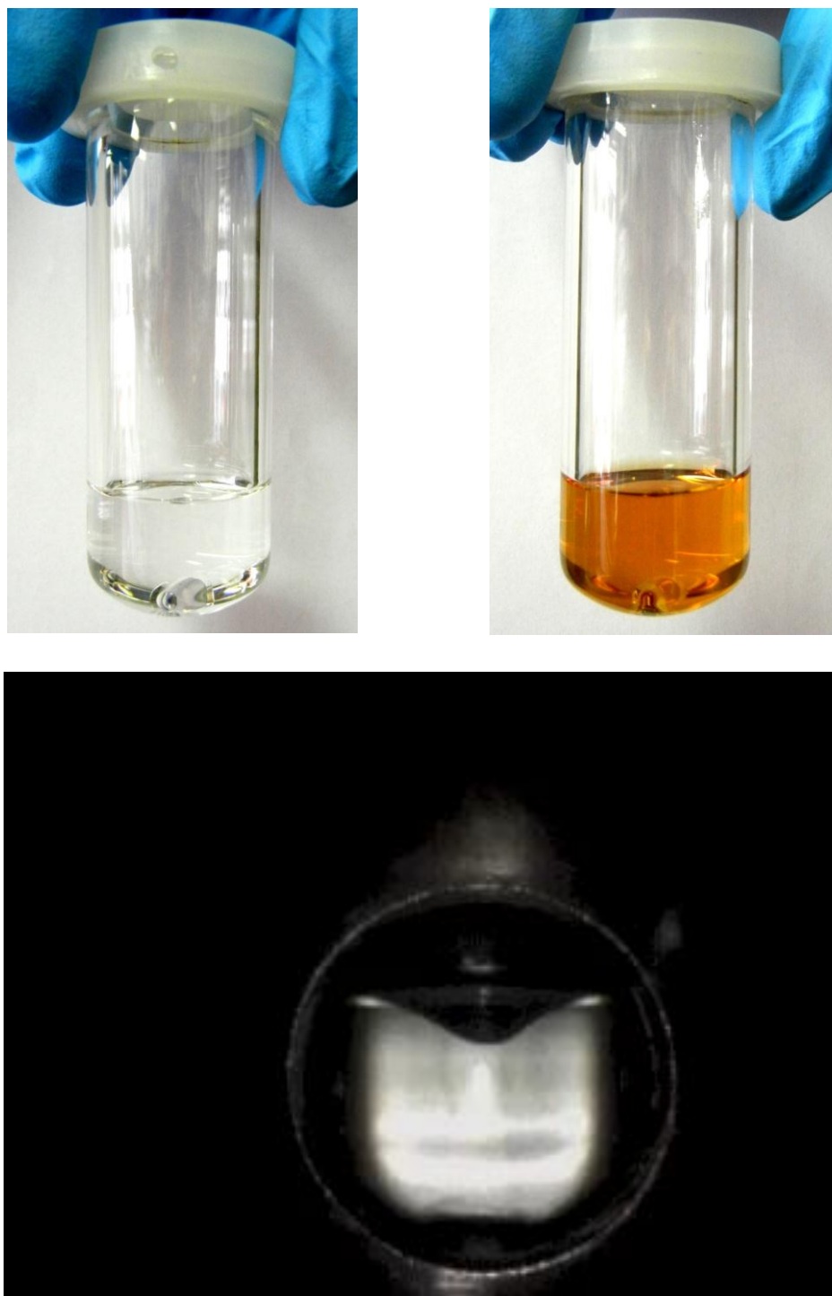
Figure 2: Upper trace: Photograph of an indium and zinc precursor mixture before (above left) and after microwave synthesis (above right); Lower trace: Real time video sequence showing the formation of the stable IZO suspensions using microwave irradiation at 140°C. The video can be downloaded.
