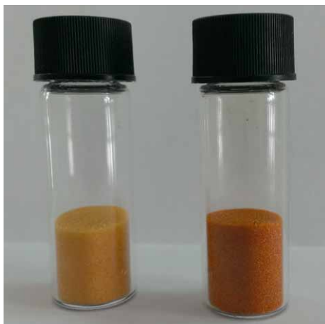
Fig. S1. Left- catalyst A (silica supported TEMPO); Right- catalyst B
