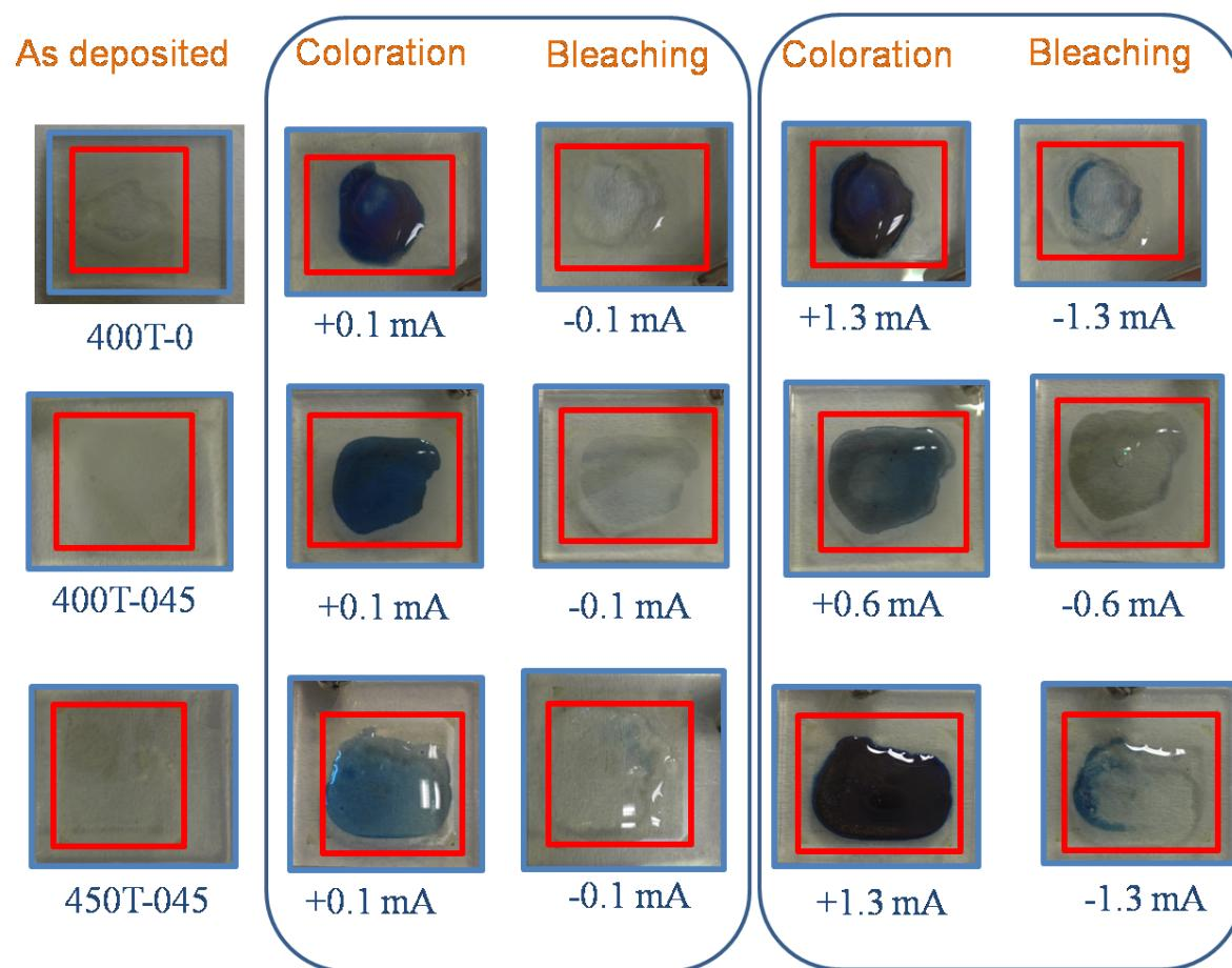
**Fig. S1** Photographs of the as deposited (bare) tungsten oxide (400T-0, 400T-045 and 450T-045) films and colored and bleached films under application of external bias, taken outside the electrolytic cell (not to the scale). For 0.1mA current the recovery of the EC properties is superior compared to other higher current values.
