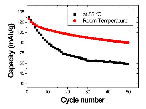
S1: Cycling performance of pristine LiMn<sub>2</sub>O<sub>4</sub> at both room temperature and 55 °C.
