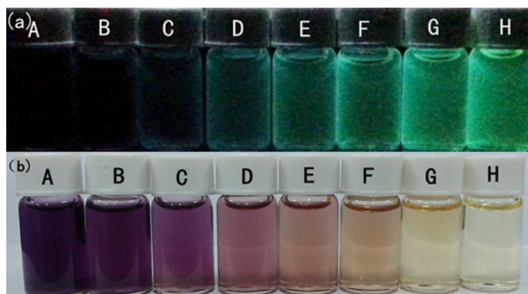
Fig. S5 From left to right (A-H) are photographs under fluorescence and visible light of Phc(10 \mu M) with the addition of CN - (0-3.5 equiv.; 0 equiv., 0.5 equiv., 1 equiv., 1.5 equiv., 2 equiv., 2.5 equiv., 3 equiv., 3.5 equiv.).
