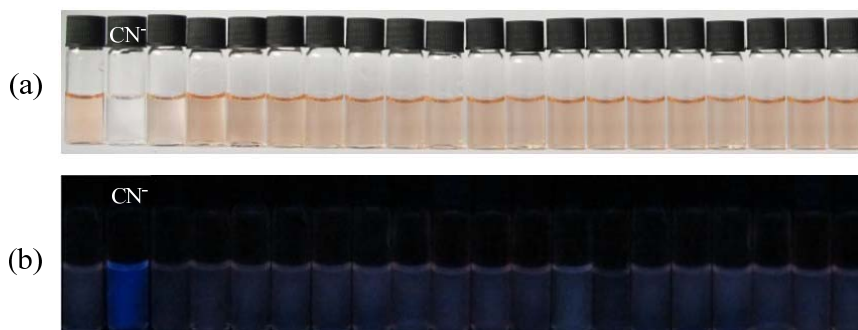
Fig. S5 (a) Color changes and (b) fluorescence color changes under a 365 nm UV light of probe 1 (20 \mu\text{M} ) with 100 \mu\text{M} of different anions (from left to right: none, \text{CN}^- , \text{S}^{2-} , Cys, \text{F}^- , \text{I}^- , \text{SCN}^- , \text{SO}_4^{2-} , \text{NO}_3^- , \text{HSO}_4^- , \text{N}_3^- , \text{Cl}^- , \text{NO}_2^- , \text{Br}^- , \text{N}_3^- , \text{H}_2\text{PO}_4^- , \text{HCO}_3^- , \text{PO}_4^{3-} , \text{CO}_3^{2-} and \text{ClO}_4^- MeOH-Tris-HCl buffer (10 mM, pH = 9.3, 1 : 1, v/v) at room temperature.
