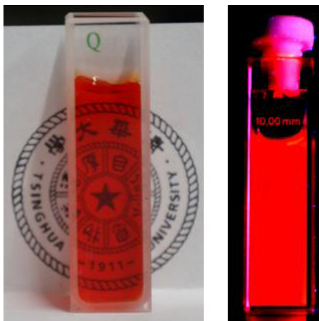
Fig. S1 Optical images of \text{PhNH}_2\text{-OA-Glu} FONs water water for more than one week. Insets are optical images of \text{PhNH}_2\text{-OA-Glu} FONs in water under UV lamp ( \lambda = 365 \text{ nm} ).
