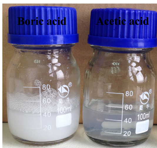
Fig. S3 Photographs of the solution after reaction at 40 °C for 80 h. The samples are prepared by using CTAB (0.02 g) and P123 (0.1 g) as template and TEOS (0.5 mL) as the silica precursor in different acidic medium (boric acid and acetic acid) at the pH value of 3.
