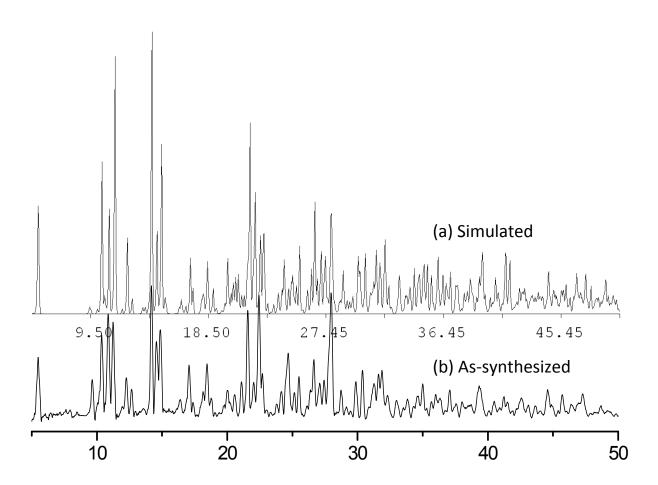
**Fig. S3** X-Ray powder patterns for **3**: (a) calculated on the basis of the structure determined by single-crystal X-ray diffraction. (b) X-ray diffractograms of an original sample of **3**.
