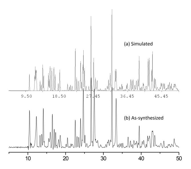
**Fig. S2** X-Ray powder patterns for **2**: (a) calculated on the basis of the structure determined by single-crystal X-ray diffraction. (b) X-ray diffractograms of an original sample of **2**.
