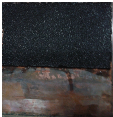
SFig.4 Digital image of Cu electrode adsorbed graphene obtained in electrochemical by direct current voltage applied
