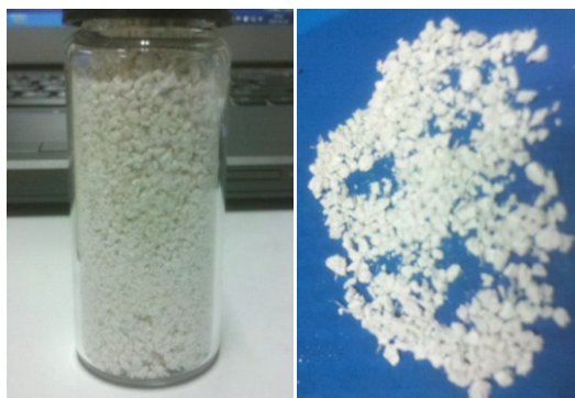
Fig. S3 The commercial product of PEEK particle with an average diameter of 500 \mu\text{m} .
