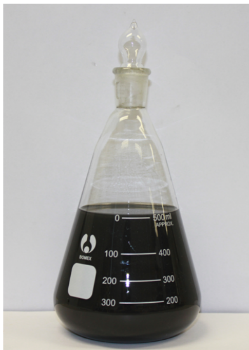
Fig. S3. Digital image of a graphite nanoflakes/DMF solution ( 10 \text{ mg mL}^{-1} ) after the ball milling and short-time sonication processes.
