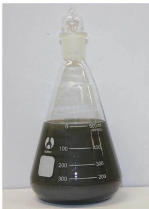
Fig. S2. Digital image of a WS 2 nanoflakes/DMF solution (10 mg mL -1 ) after the ball milling and short-time sonication processes.
