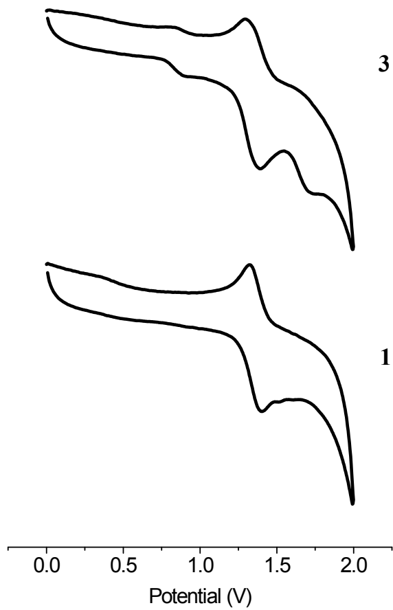
Figure S13. Cyclic voltammogram of 1 (bottom) and 3 (top) on a glassy carbon millielectrode in CH 3 CN (Et 4 NClO 4 ) versus Ag/Ag + at 25 °C.
