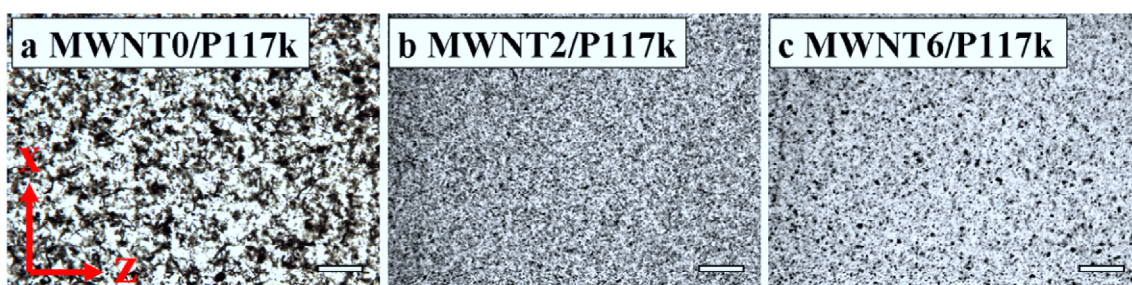
Fig. S23 Structures of 0.5 wt % MWNT0/P117k (a), 0.5 wt % MWNT2/P117k (b) and 0.5 wt % MWNT6/P117k (c) under a shear rate of 0.01 \text{ s}^{-1} . The scale bars are 150 \mu\text{m} and the gap is 150 \mu\text{m} . Photos are taken after shearing for about 45 s.
