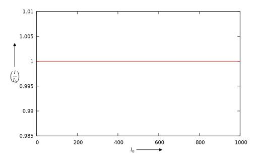
The above simulation shows the variation of normalized peak intensity in the LLC spectrum as a function of no of loops " $l_0$ " indicated in the sequence. It shows complete absence of any modulation in a weakly coupled spin-1/2 system. Relaxation is not included in the above simulation.
