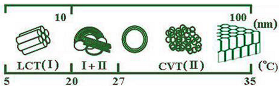
Scheme S1 Evolution of siliceous structures with different pore diameters as a function of synthesis temperature when the other reaction conditions are exactly the same. The illustrated models are not to scale.
