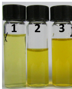
Figure S3: Photographs of different CNDs under room light: 1, CNDs-1; 2, CNDs-1-Cys; 3, CNDs-1- \text{Na}_2\text{S} .
