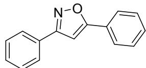
White solid; yield: 75%; m. p. 140-142 °C; <sup>1</sup>H NMR (400 MHz, CDCl<sub>3</sub>, ppm): δ 7.86 (m, 4H), 7.49 (m, 6H), 6.84 (s, 1H); <sup>13</sup>C NMR (CDCl<sub>3</sub>, 125 MHz): δ 168.7, 161.3, 128.6, 128.4, 127.4, 127.3, 127.3, 125.8, 125.1, 124.2, 95.8; IR (CHCl<sub>3</sub>): ν<sub>max</sub> 3437, 3114, 2924, 1462, 1257, 1092, 763 cm<sup>-1</sup>; ESI-MS: *m/z* 222.08 [M+H]<sup>+</sup>; HR-ESIMS: *m/z* 222.0917 calcd for C<sub>15</sub>H<sub>11</sub>NO+H<sup>+</sup> (222.0913).
