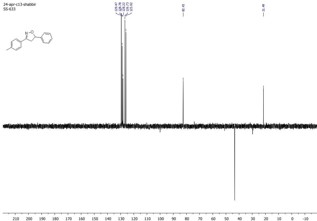
S3.19.  $^1\text{H}$ ,  $^{13}\text{C}$ , and DEPT135 NMR spectra of 5-phenyl-3-(o-tolyl)-4, 5-dihydroisoxazole (**6g**)
