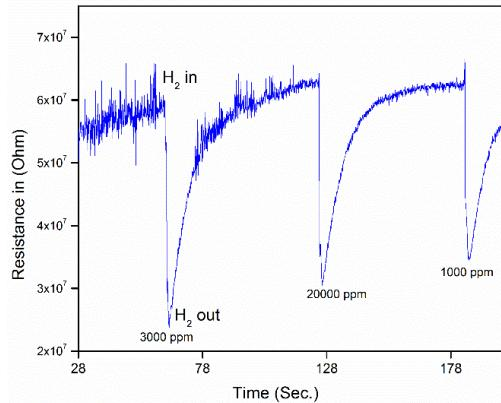
**Figure 1:** Gas sensor response of ZnO/zeolite nanocrystals for different hydrogen gas concentrations.
