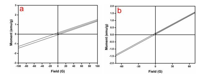
**Fig. S3.** Coercivity of collagen fibers treated with IOOANP in M-H curve probed using a vibrating sample magnetometer.
