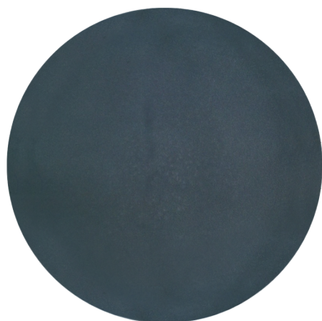
Figure S8. Large Ti/TiO 2 -nanotubes/PbO 2 anode in disk format before its use to treat a synthetic dye effluent by electrochemical oxidation.
