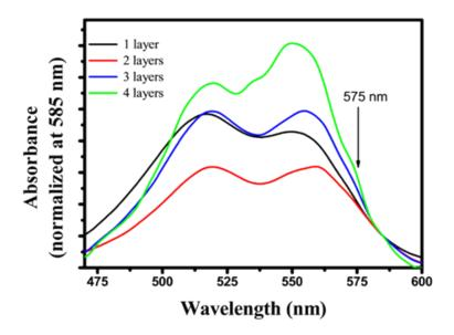
**Fig. S1.** Normalized UV-Vis absorption spectra of  $\{PEI/GO/PEI/PSS/PyY/PSS\}_n$  multilayer film at various layers.
