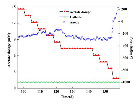
Fig. S4 Anode and cathode potential at various acetate dosages in BC-BES.
