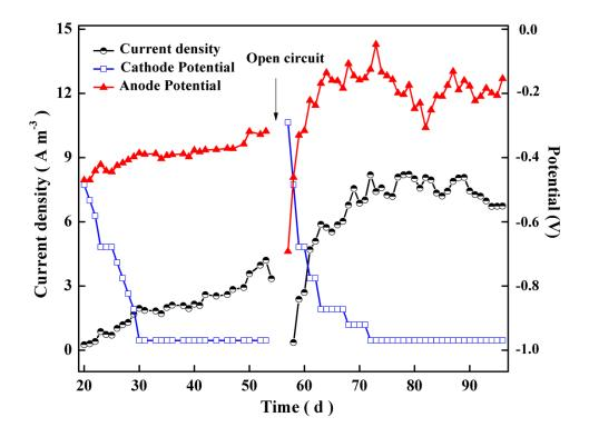
Fig. S1 Anode potential, cathode potential and current density in BC-BES.
