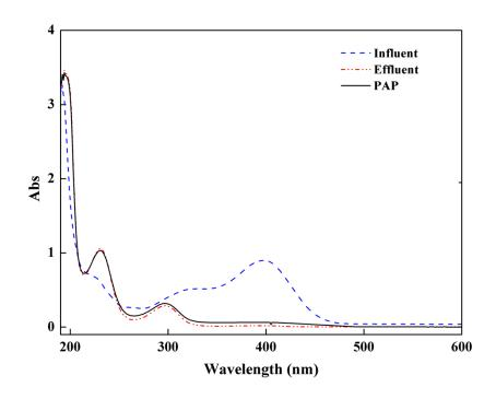
Fig. S2 Evolution of UV-vis spectra for PNP reduction and PAP formation in BC-BES.
