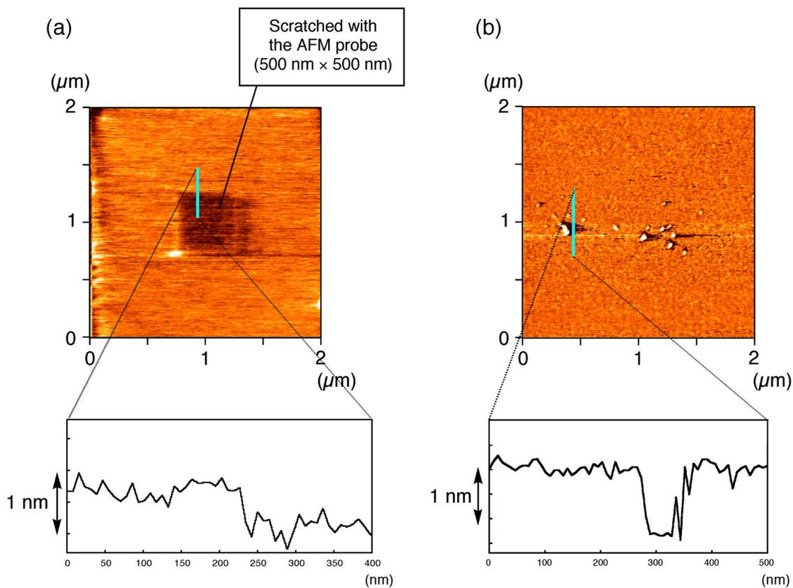
**Fig. S2** Examples of the AFM images used to examine the film thickness: (a) compound **1** transferred at  $5 \text{ mN m}^{-1}$ ; (b) compound **2** transferred at  $10 \text{ mN m}^{-1}$ .
