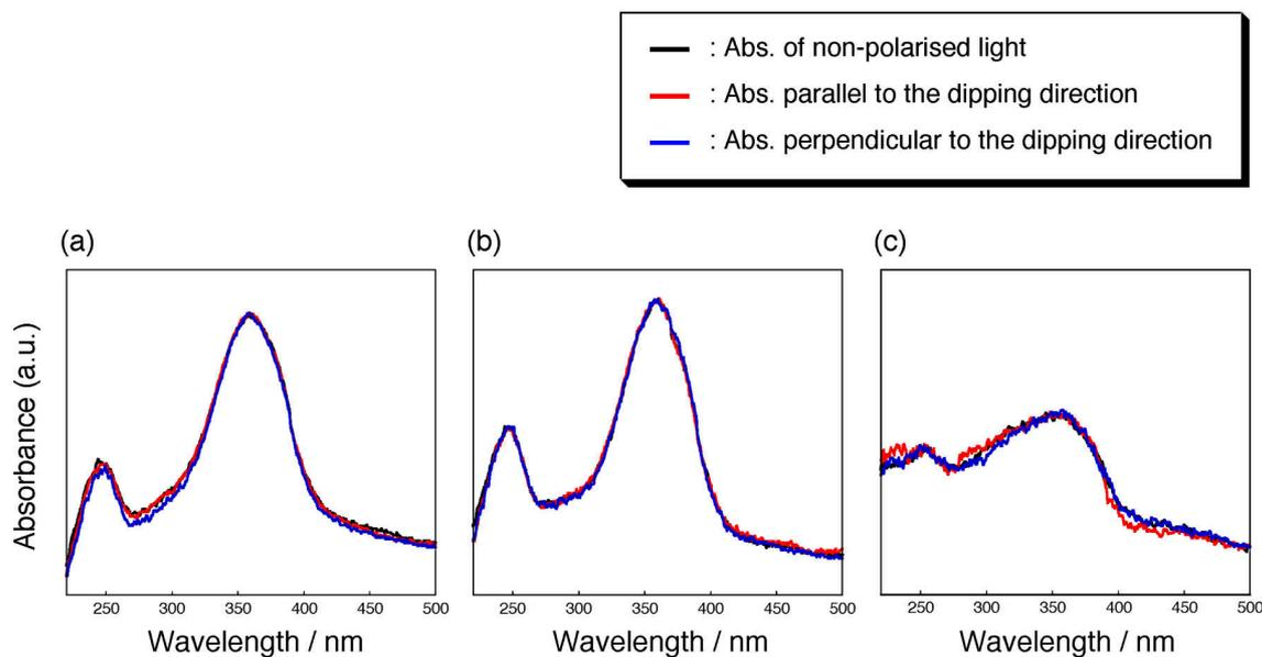
**Fig. S1** UV/Vis spectra of the LB film of **2** transferred at the surface pressure of  $30 \text{ mN m}^{-1}$  onto a quartz substrate: (a) after deposition from the water surface; (b) LB film exposed to polarised visible light ( $436 \text{ nm}$ ,  $1000 \text{ mJ cm}^{-2}$ ); (c) LB film exposed to  $30 \text{ mJ cm}^{-2}$  of polarised UV light ( $365 \text{ nm}$ ).
