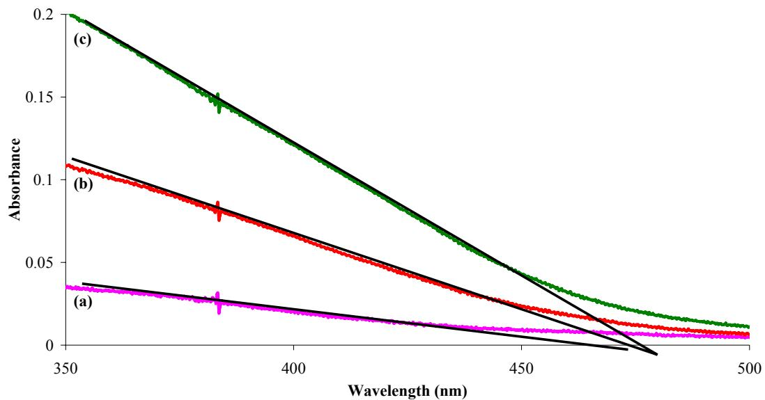
**Figure S3.** UV-Vis absorption edge profiles for CdS/clathrin constructs prepared at constant clathrin concentration but with CdS : clathrin molar ratios of (a) 3870, (b) 6450 and (c) 12900, corresponding to CdS particle sizes of 5, 6 or 7 nm, respectively.
