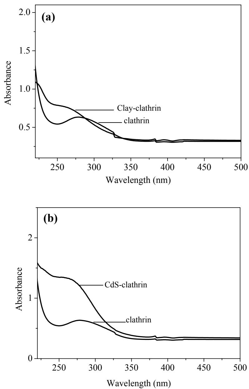
**Figure S2.** UV-Vis spectra for (a) unmineralized clathrin cages, and organoclay- or organosilica-coated clathrin cages, (b) unmineralized clathrin cages and CdS-decorated constructs.
