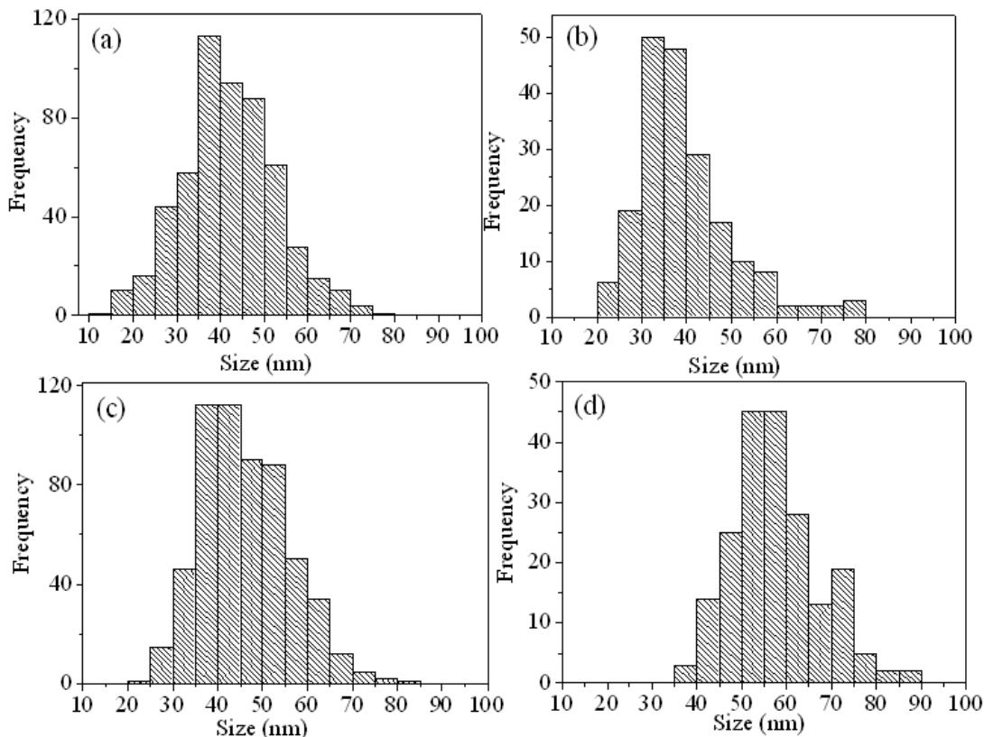
**Figure S1** Particle size histograms for (a) unmineralized clathrin cages, and clathrin cage/inorganic nanoparticles prepared in the presence of (b) organoclay clusters, (c) organosilica oligomers, and (d) CdS.
