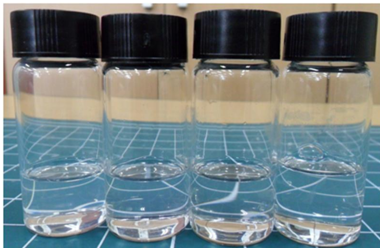
Fig. S1 Stability of the PVCFeS-SiSH metallopolymer solutions of various ratios (0.01, 0.05, 0.1 and 0.2 phr) of SiSH, which have been stored at room temperature for 6 weeks.
