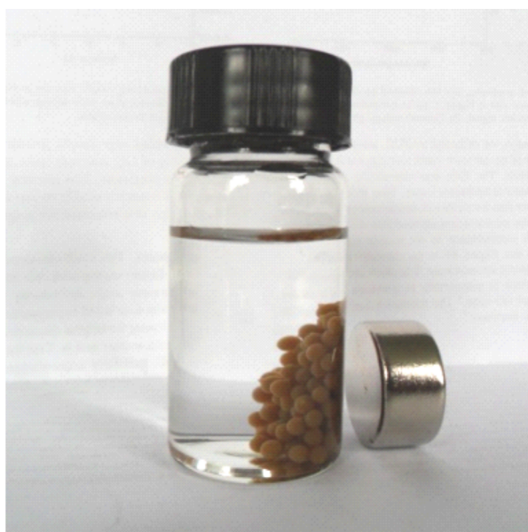
Fig. S2. Photograph for the magnetic separation of the beads from solution under an external magnetic field.
