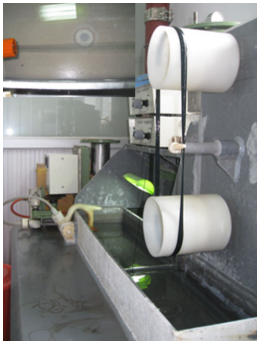
Fig. S1 Photographs of fiber spinning from PANI/cellulose solution via a simplified laboratory spinning frame.
